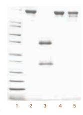
50 mM TCEP, but not DTT, prevents IgG oxidation and aggregation in unattended samples. Electrophoresis pattern of human IgG using sample buffer with TCEP or DTT as the reducing agent. 2X sample buffers were left at room temperature for four weeks. Each day the tubes containing the buffer were left open for 15 - 30 minutes to mimic everyday use. Lane 1. Molecular weight markers. Lane 2, 3, 4, 5: four-week old sample buffer containing 10 mM TCEP, 50 mM TCEP, 10 mM DTT or 50 mM DTT, respectively.
