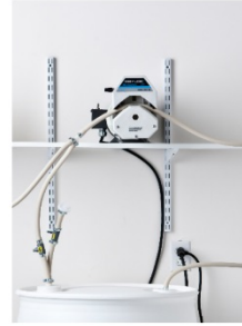
Step #3 - Connect Pump to center hose
